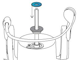
A thicker washer stack will place more line to the rear of the spool. If your line skewed towards the top of the spool. Add the thin washer included with the reel.
