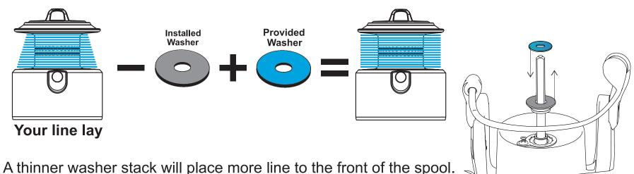
If your line is skewed towards the bottom, remove the washer that is already installed and replace with the washer included with the reel.
